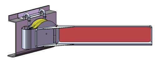
The floating, self-supporting, water and oil directing containment boom, which is installed at a 45 degree angle to the collector, is light and easy to attach. The length of the containment boom can be adjusted, as needed, from 2 metres to 3 metres.
