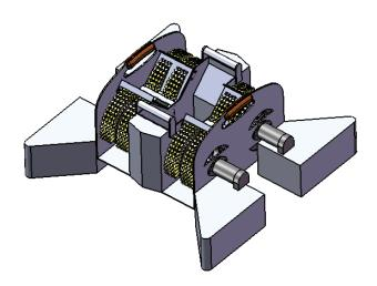
The oil collection station can be removed for cleaning and for changing brushes, depending on the different qualities of oil.
